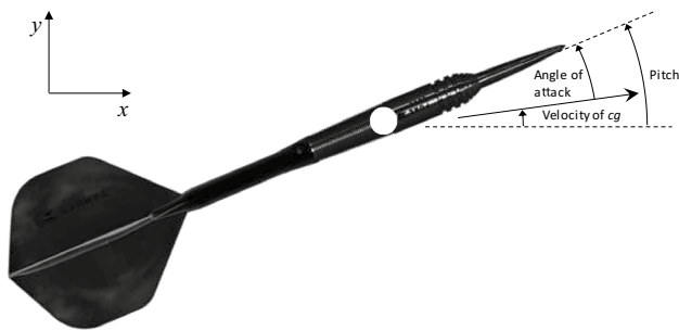
Fig. 3 A schematic of the dart's dynamic parameters
