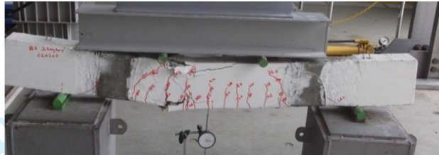
(b) Rupture of GFRP with concrete crushing failure of beam FSB-CA2
