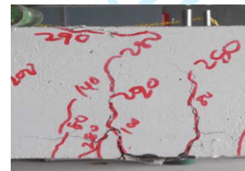
(b) Rupture of GFRP with concrete crushing failure of beam FSB-UA2
