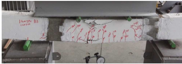
(a) Rupture of GFRP with concrete crushing failure of beam FSB-CA1
