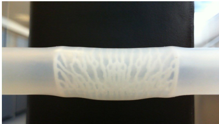
Figure 5-11: Stent inserted in to the inflated artery.
