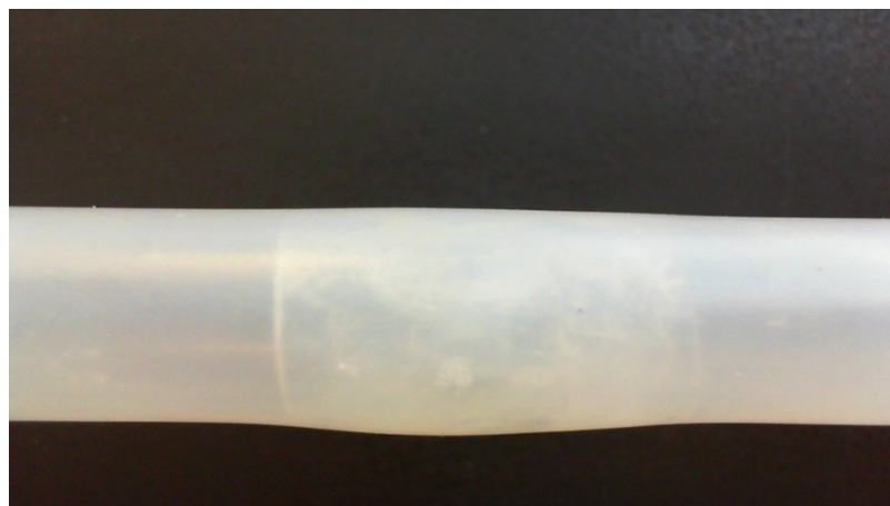
Figure 5-15: Simulated plaque added to the mock artery with the thickest part at the bottom.
