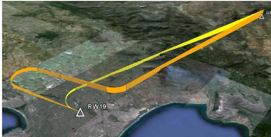
Figure 2-17 Example of Reduction of Flown Distance between Conventional (orange) and RNP (yellow) operations (Airbus, 2015).
