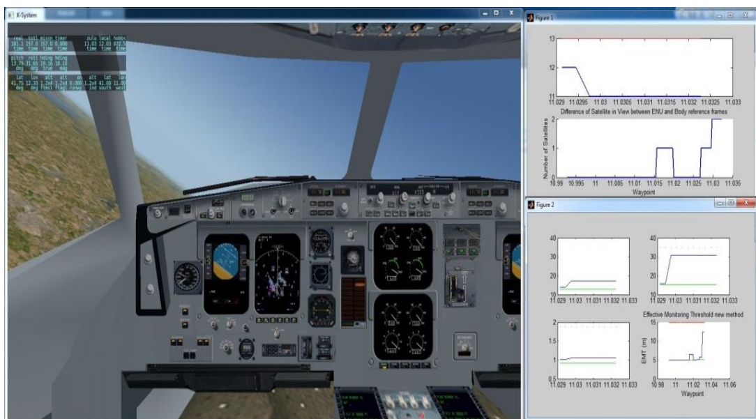
Figure 6-1 Real-time ARAIM computation integrated in the X Plane software.
