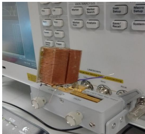
Figure 4.25- The two port network measurements of two inductors on short substrate
