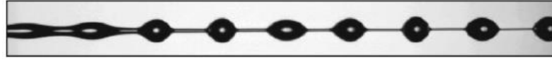
Figure 32: Example of a beads-on-a-string jet caused by the high extensional viscosity of the polymeric additives of the ink (50/50 water-glycerol + 0.05 % 1 MDa poly(ethylene oxide)). Image from (Christanti & Walker 2002).
