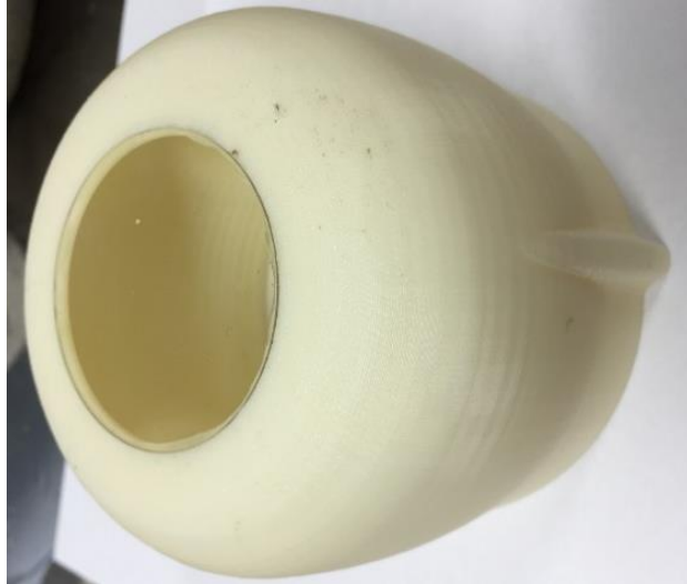
Figure 2.14: Custom made protective casing with the transparent window for HGC.
