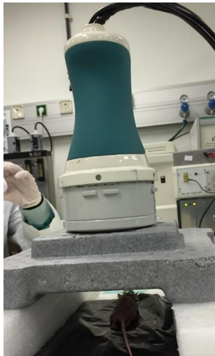
Figure 4.14: Photograph of the animal imaging setup at Leiden University Medical Centre using Nebuleye. The camera was positioned on an ad-hoc foam stand to minimise motion effect during image acquisition.
