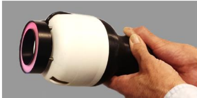
Figure 9.2: Laboratory prototype of a co-aligned gamma-NIRF imaging system modified using HGC with an addition of a bandpass filter and a LED ring as the excitation light source. Image courtesy of University of Leicester.
