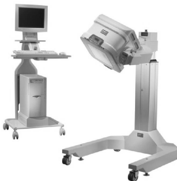
Figure 1.11: A mobile gamma camera-Mediso 'Nucline™ TH' (Taken from [13]).
