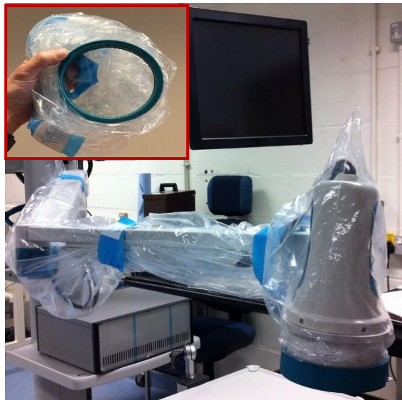
Figure 2.23: The sterile drape fitted on the Nebuleye. (Inset) Clear cap window to allow production of the optical image.
