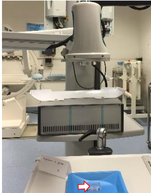
Figure 3.6: Experimental set up for the intrinsic uniformity test. A ^{99m}\text{Tc} point source (arrow) was placed underneath of the Nebuleye with the collimator removed.
