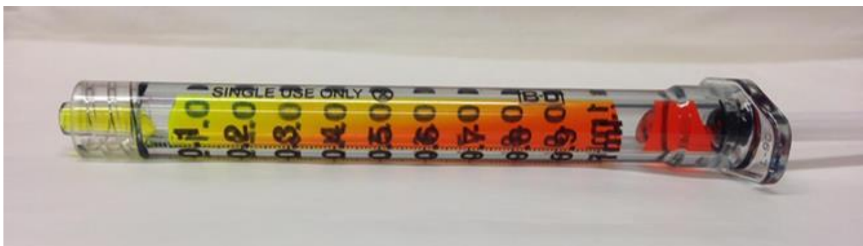
Figure 2: Colour photograph showing the lack of mixing and dead space in a 1ml syringe, illustrated by drawing up a minim of Fluorescein and 0.5ml of water for injection.
