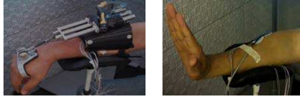
Fig. 2: The setup of the EMG sensors on the forearm, with and without the orthosis.
