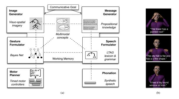
Figure 6: (a) Schematic of the generation model for speech and iconic gesture; (b) exampe utterances produced with it.
