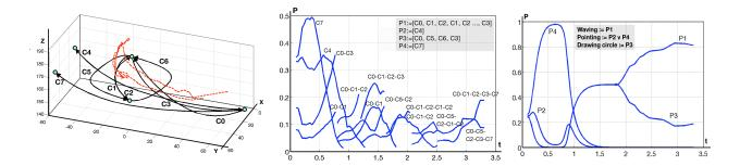
Figure 4: Example of probablistic gesture perception of a waving gesture (dotted; *left*) with the evolving probabilities of the agent's own corresponding motor commands (*middle*) and motor programs (*right*). The motor program **P1** is eventually singled out already during observation.
