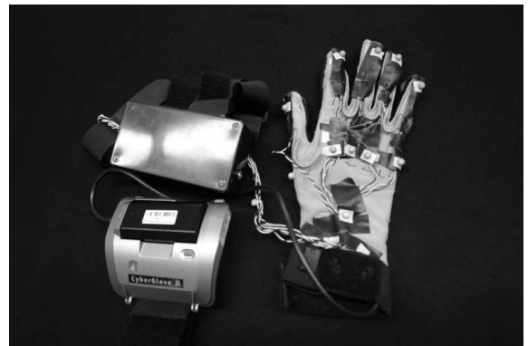
Figure 3. CyberGlove with 11 VICON markers; five markers are situated on the fingertips, five markers on the knuckles and one marker on the back of the hand.
