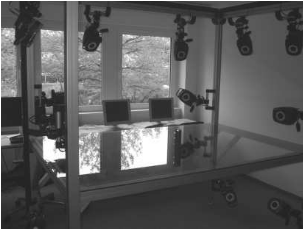
Figure 1. 14-camera VICON setup: the cameras are situated on both sides of the transparent glass table.
