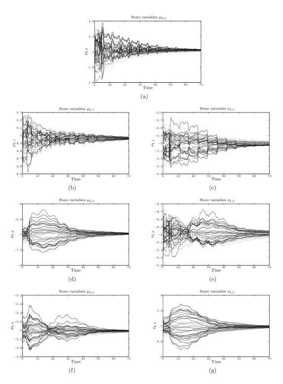
Fig. 3.4: Time evolution of  $\mu_{k,0}$  (Figure 3.4(a)),  $\mu_{k,1}$  and  $\nu_{k,1}$  (Figures 3.4(b) & 3.4(c)),  $\mu_{k,2}$  and  $\nu_{k,2}$  (Figures 3.4(d) & 3.4(e)) and  $\mu_{k,3}$  and  $\nu_{k,3}$  (Figures 3.4(f) & 3.4(g)) for 39 PSSs, interacting through the network in Figure 3.2(a).
