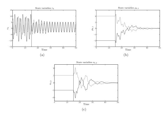
Fig. 3.8: Time evolution of  $r_k$  (Figure 3.8(a)),  $\mu_{k,1}$  (Figure 3.8(b)) and  $\nu_{k,2}$  (Figure 3.8(c)) for two PSSs. Coupling dynamics and adaptive mechanisms are switched on at t = 15 (black solid line).
