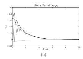
Fig. 2.2: Time evolution of  $\omega_k$  (Figure 2.2(a)) and  $\rho_k$  (Figure 2.2(b)) for four HOPF oscillators, interacting through the network in Figure 2.1. In both figures, all variables converge towards a constant and common consensual value.
