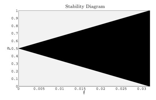
Fig. 5.2: Stability diagram for parameters f and p for the System (5.8) with discrete stochastic switching F(t). The stable region is given in black, the unstable regions in gray.
