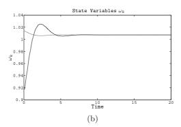
Fig. 2.4: Time evolution of  $r_k$  (Figure 2.4(a)) and  $\omega_k$  (Figure 2.4(b)) for two Hopf oscillators. The two oscillators manage to adapt their frequencies while their radii do not converge towards their respective attractor.
