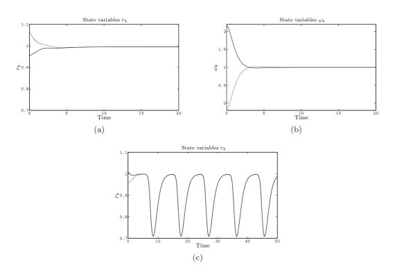
Fig. 4.6: Time evolution of  $r_k$  and  $\omega_k$  for two heterogenous  $q_k$ -DVSs with adapting frequencies (Figure 4.6(a) & 4.6(b)), and time evolution of  $r_k$  for two heterogenous  $q_k$ -DVSs with no adaptation (Figure 4.6(c)).
