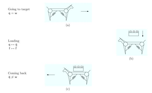
Fig. 4.2: The robot dog on its way to collect the box of bottles (Figure 4.2(a)) - value of w set to q, guaranteeing maximum leg stride. The box of bottles is loaded on the robot dog's back (Figure 4.2(b)) - change in values of  $q \mapsto \check{q}$  and  $f \mapsto \check{f}$ . The robot dog comes back (Figure 4.2(c)) - value w does not equal new value  $\check{q}$ , maximum leg stride is no longer attained.
