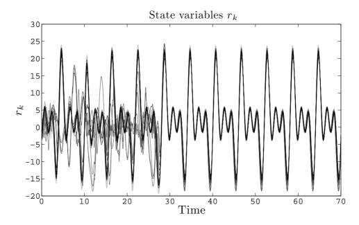
Fig. 3.7: Time evolution of  $r_k$  for 39 PSSs with all their adaptive mechanisms switched off (i.e. all susceptibility constants are zero), interacting through the network in Figure 3.2(b).
