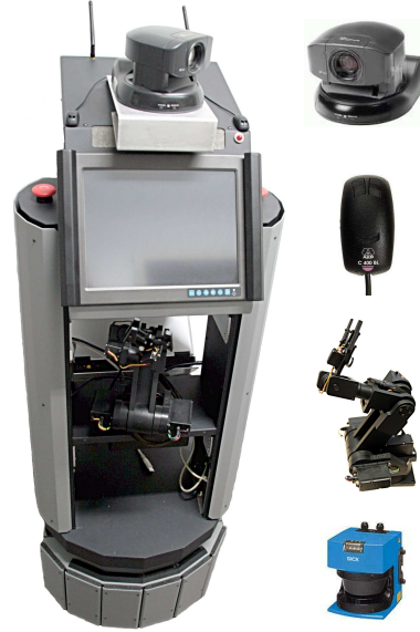
Fig. 1. The robot ToBI with its components shown on the right. From top right: Pan-/Tilt-camera, interfacial microphone, Pioneer 5DOF arm and laser range finder.
