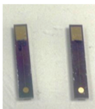
Fig.1. Comparison of colour changes observed at 1 mm gold disc electrode surface on an unmodified electrode (left) and on electrode after sol-gel electrodeposition (right)
