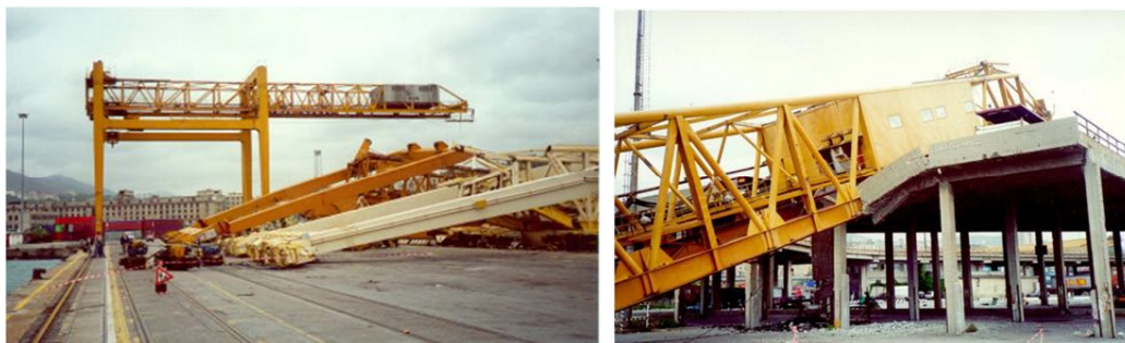
Figure 3. Consequences of the downburst occurred in the Port of Genoa on 31 August 1994
