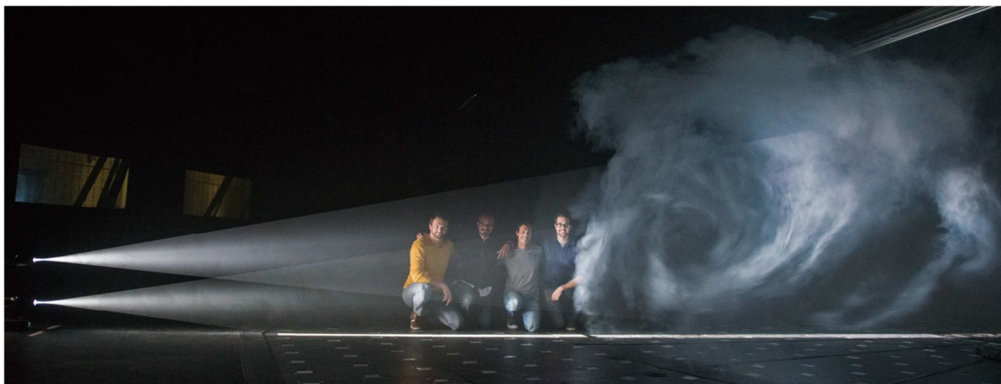
Figure 13. Wind tunnel simulations at WindEEE, UWO (courtesy Prof. Horia Hangan)
