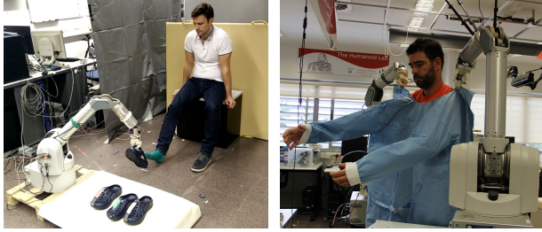
Figure 1: Robot assisted-dressing tasks developed under the I-DRESS project. The assistance with putting on a shoe shown on the left is an example of a single-arm robot task, and it is intended for users with reduced mobility. The assistance with gown dressing shown on the right is a dual-arm robot task and represents the case of medical staff whose physical contact with the garments must be limited during dressing to avoid contamination.
