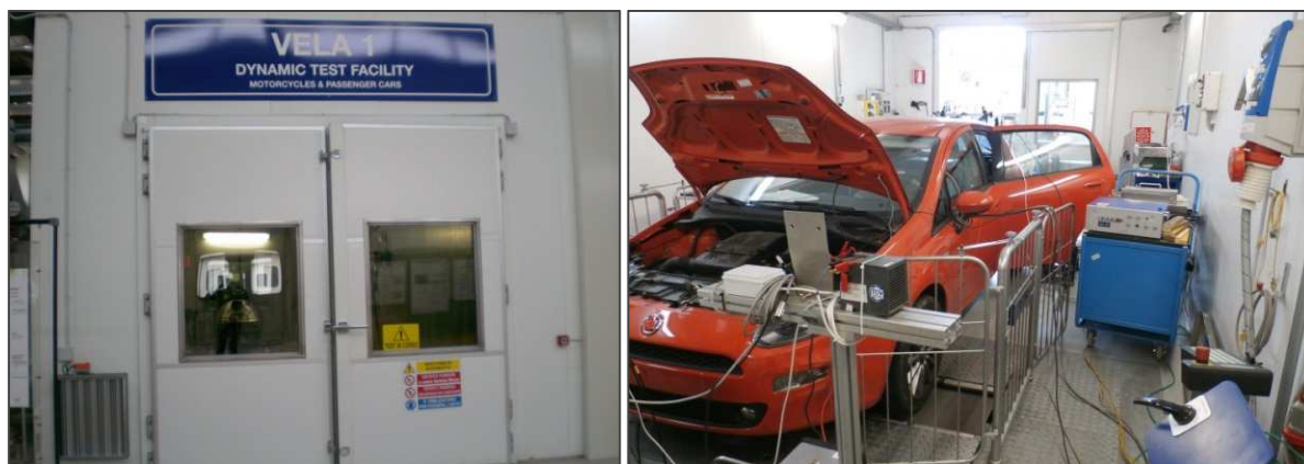
Figure 1. The Vehicles Emissions Laboratories (VELA) test cell at JRC (left) and a passenger car on the roller bench inside the test cell (right).
