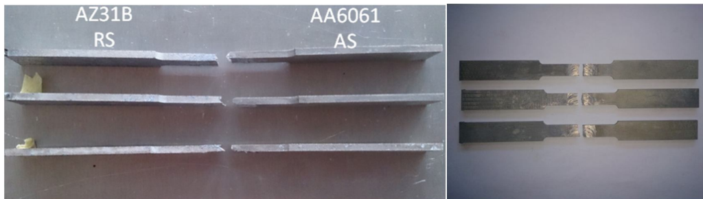
Figure 4. Tensile test comparisons between FSW welding with filler and without filler.
