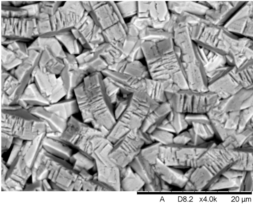
Figure 5-14a SEM photo of 10 min electroplating sample surface(4000)
