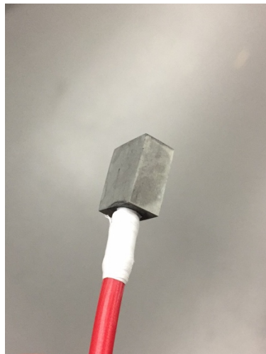
Figure 5-6 Electroplated sample using zinc sulfate, potassium pyrophosphate solution
