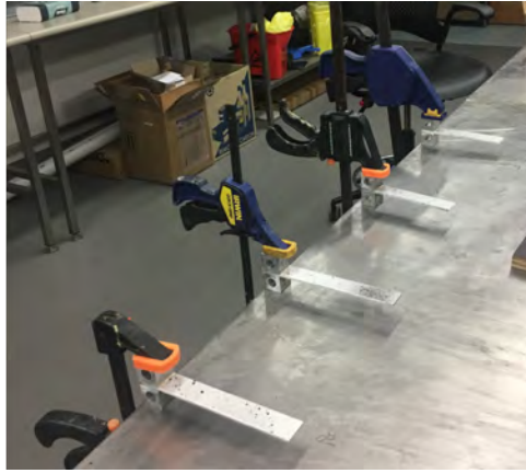
Figure 3.11: Clamps applied to the samples to bond the loading blocks
