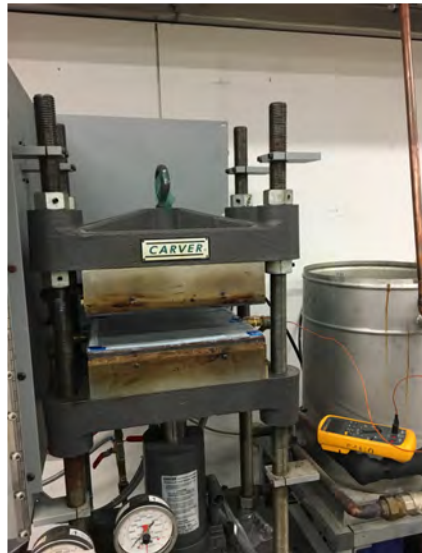
Figure 3.8: FML composite bonding in the hot-press
