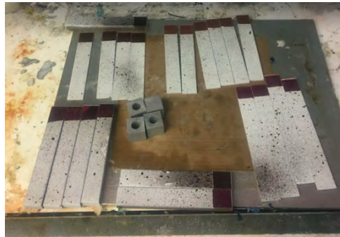
Figure 3.10: Speckle pattern applied to the samples
