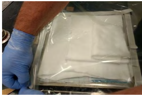
Figure 3.2: Vacuum bagging application for GFRP manufacturing
