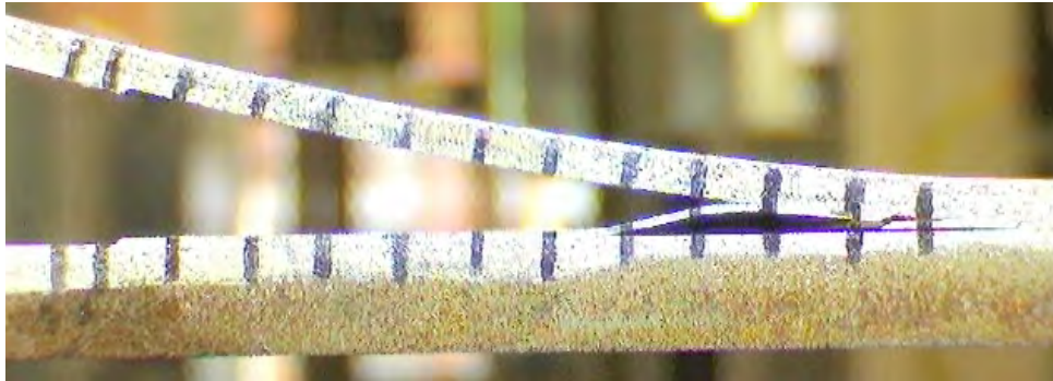
Figure 7.5: Mixed mode sample 2 exhibiting shear loading along the FML interface
