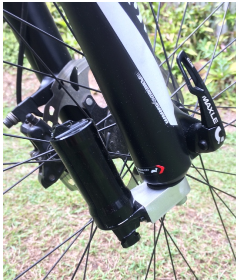
Figure 31: Prototype bottom-out damper on Rockshox Lyrik fork
