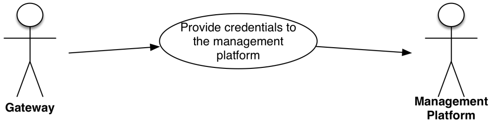
Figure 3.14: Use case diagram: Gateway authenticates itself on the platform.
