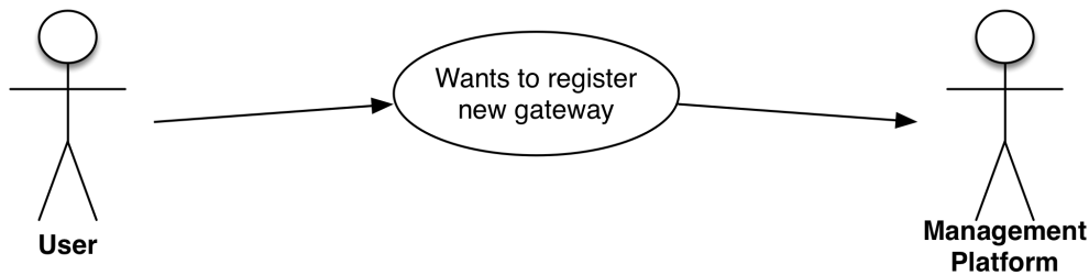
Figure 3.12: Use case diagram: User wants to register a new gateway on the platform.
