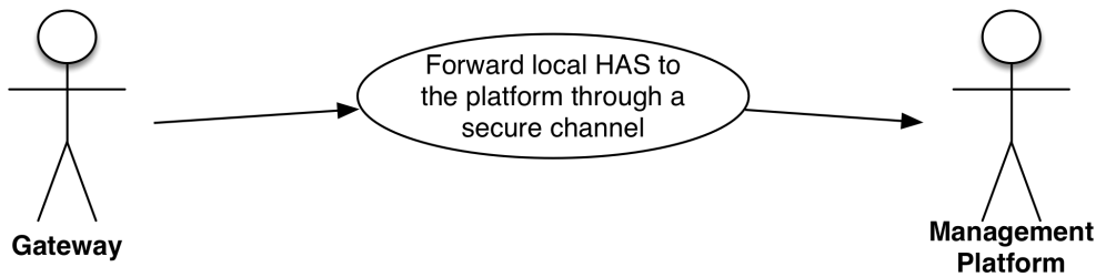
Figure 3.16: Use case diagram: Gateway forwards the HAS to the platform.
