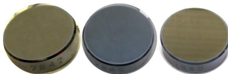
Figure 31 B 4 C-coated Si test mirrors during various stages of the process. Left: Pristine B 4 C-coated Si mirror; Center: Mirror after a-C coating (full mirror surface coated); Right: Mirror after cleaning with pure O 2 plasma.
