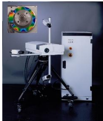
Figure 2-3 Dantec Dynamics Company apparatus, 3D Pulse ESPI system, http://www.dantecdynamics.com/Default.aspx?ID=1603
