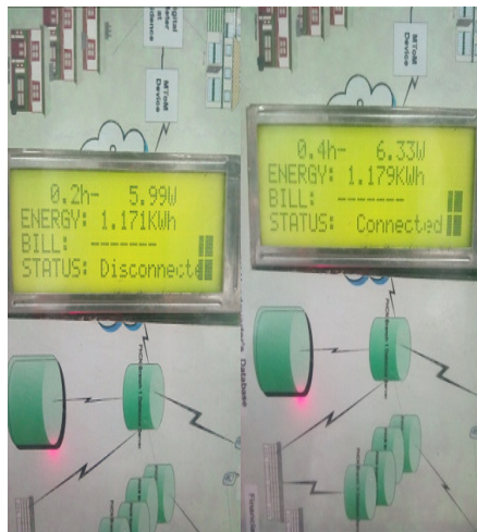
Fig. 3 The Disconnected and Connected Meter Operational State
