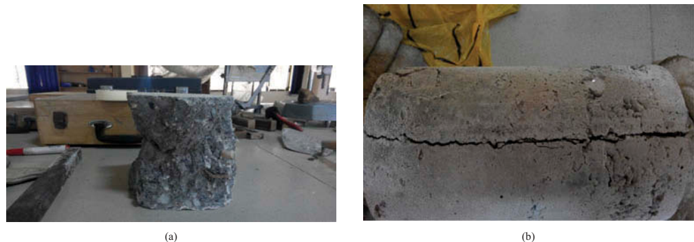
Figure 8. (a) Failure pattern of cube sample (b) Failure pattern of cylinder sample.
