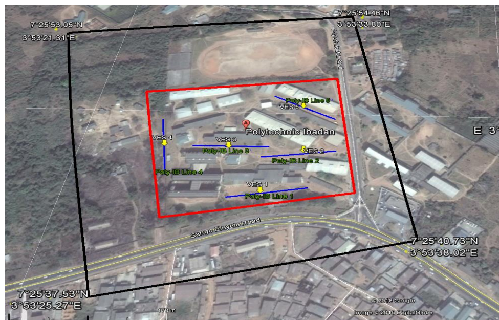
Figure 2 Satellite imagery map of the study site in Ibadan indicating the 2D resistivity profile lines (blue) and VES points (yellow arrows)
