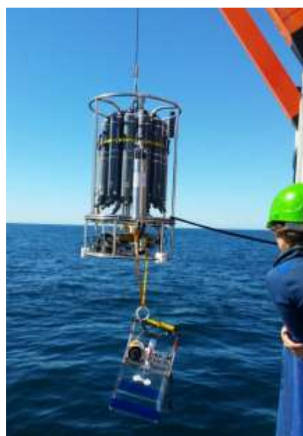
Fig. 1 Deployment of one CUBE with the CTD / water sampling instrument. (Picture: Janina Büscher)
