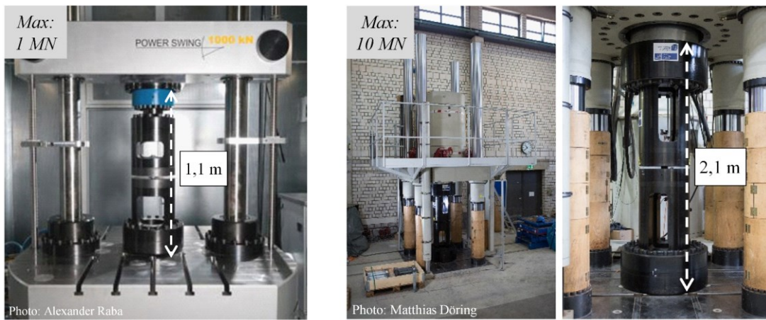
Figure 3: Test setup for fatigue tests on HV-bolt sets M36 in a high frequency pulsator (left) and for HV-bolt sets M64 high-strength servo-hydraulic testing machine (right)
