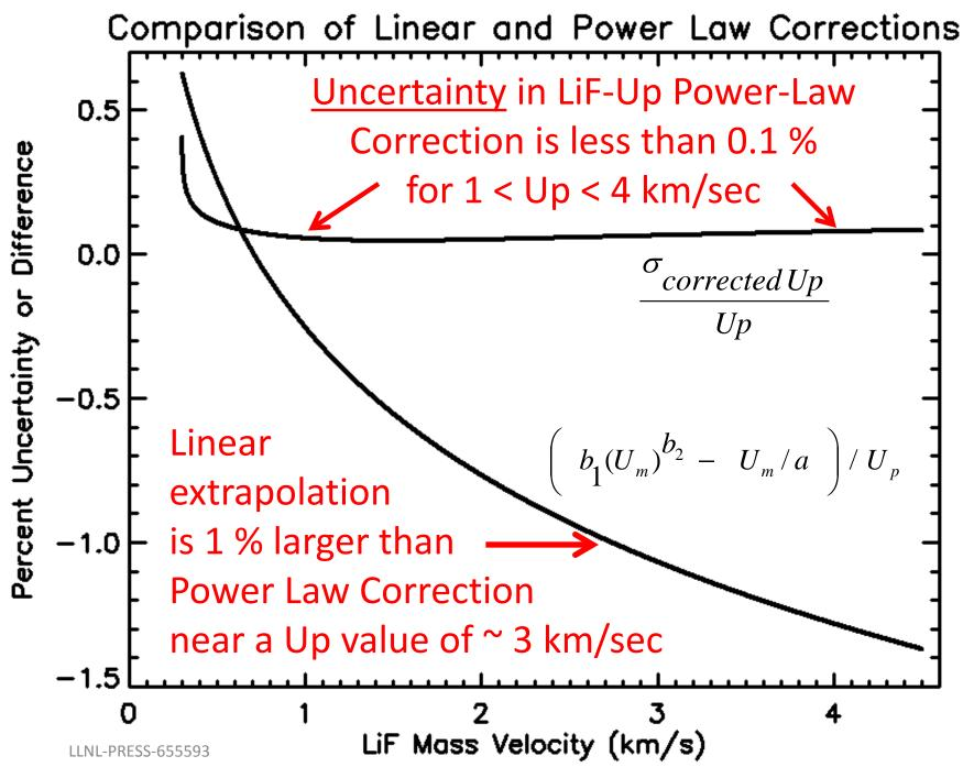
For Ta impacting Ta-LiF with release Up = 3.1 km/sec, these quantities are no larger than 0.18 %:
