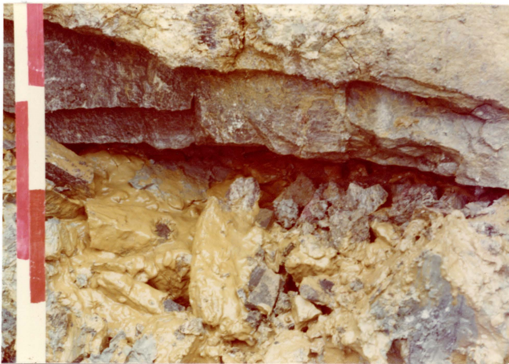
Photo 16. Liquid clay about one foot above bottom of section. Scale six inches (left) and ten centimeters (right).
