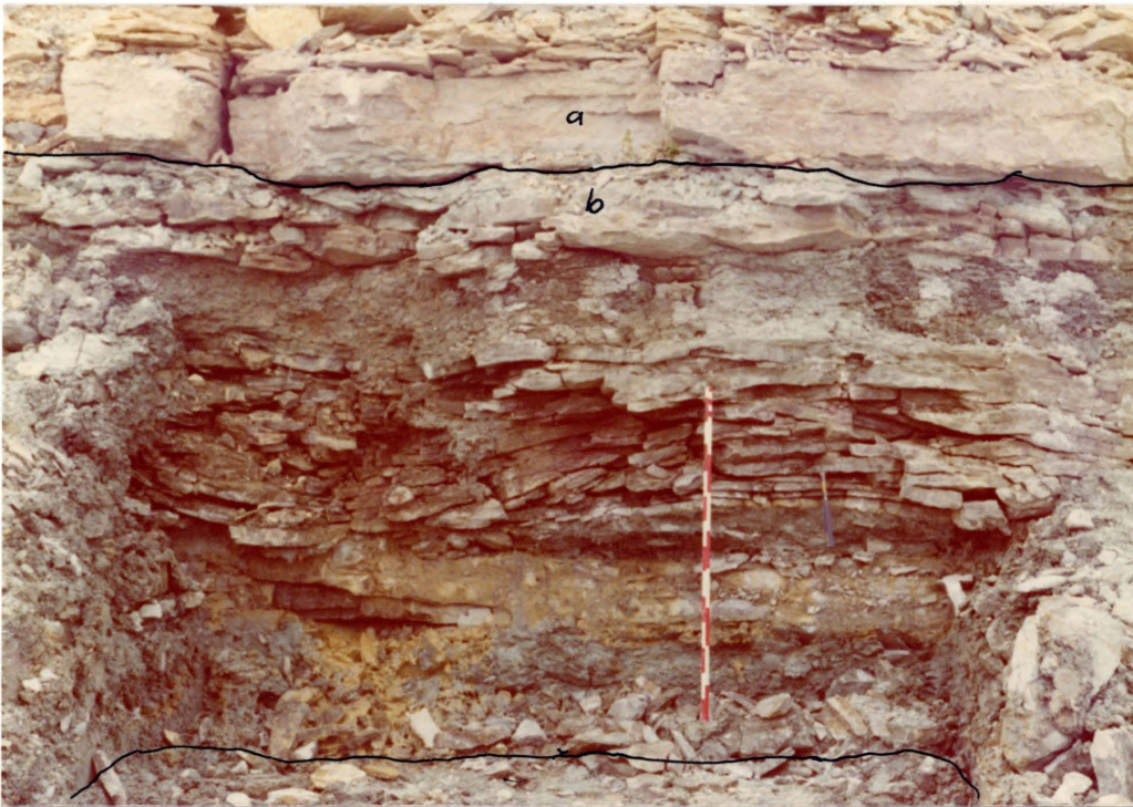
Photo 11. View of location of upper section showing Dayton Formation (a) and Brassfield Formation (b). Scale 10 centimeters (left) and six inches (right).
