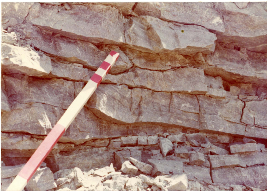
Photo 9. Cross bedded laminations about ten feet from top in lower section. Six inch scale shown.
