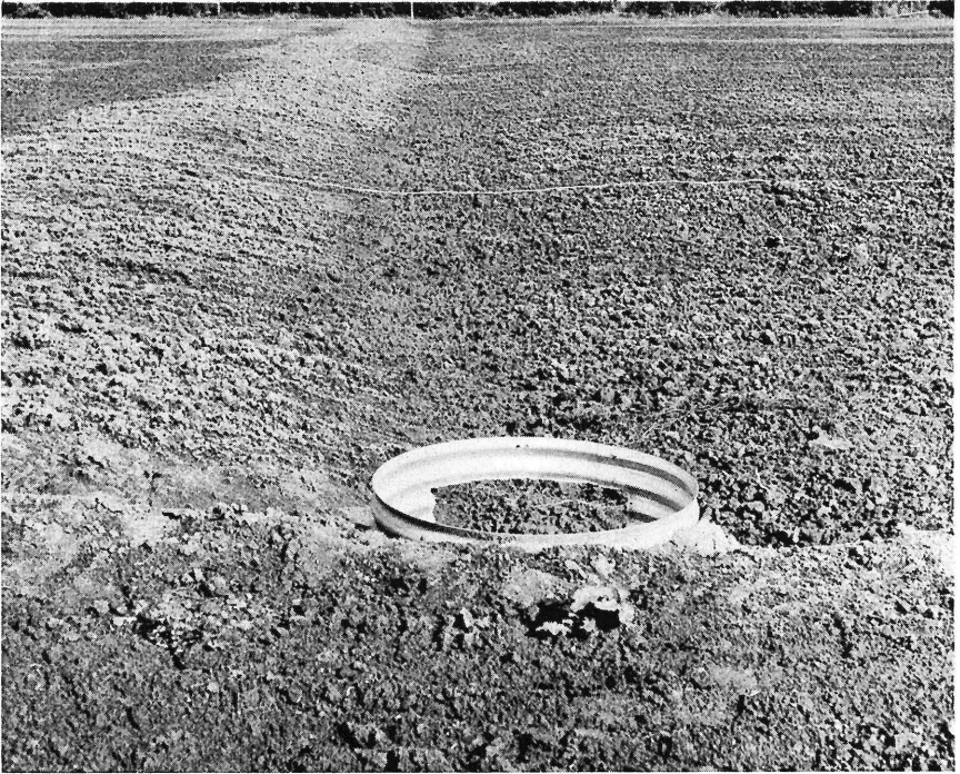
Fig. 5.—Typical surface drain in the B and D plots and earth dike between plots on the left.
