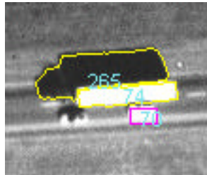
Figure 3.16 A candidate truck that matches with both region pattern model and line pattern model
