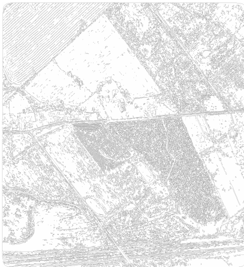
Figure 2.6 Edge detection at refined resolution ( S = 1.6 , width = 23)
