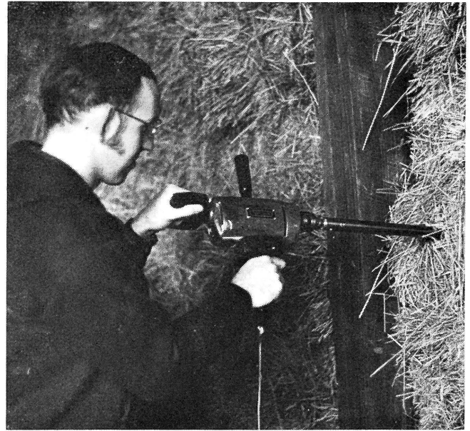
FIG. 3.—Sampling baled hay with a “Penn State Hay Sampler” and a ½ inch electric drill.
