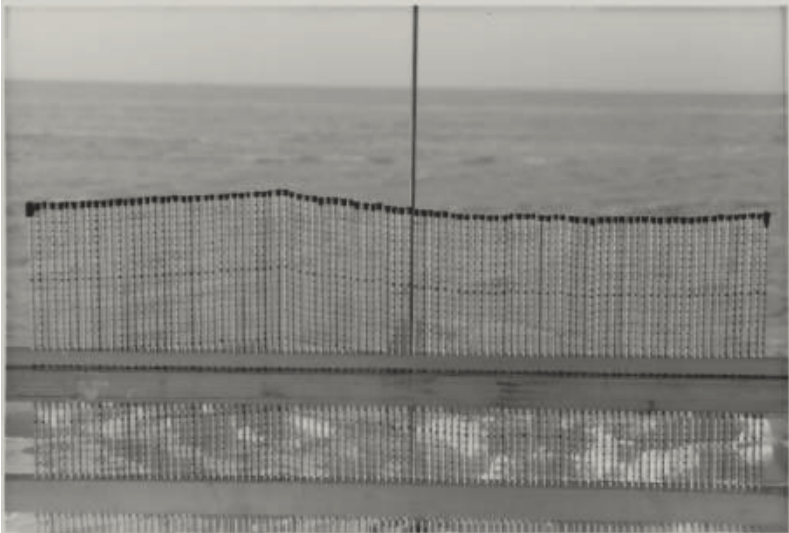
Figure 12. Rods tapped lightly through upper (~1cm) fresh snow. Page 11 in G Book. RMS Height: 0.75 cm. Correlation length 10 cm.
