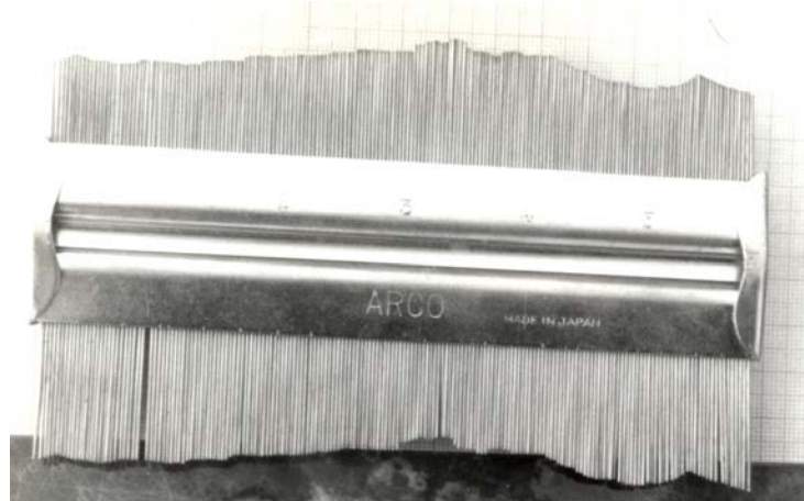
Figure 23. Ice layer surface roughness. Gauge on cm scale graph paper (above).
