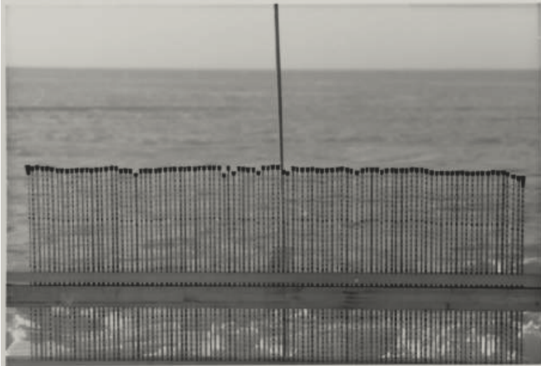
Figure 13. 'Stucco' Surface along wind field. Low rods punched through surface crust. P. 24/25 G Book. RMS Height: 0.34 cm. Correlation Length: 3.91 cm.
