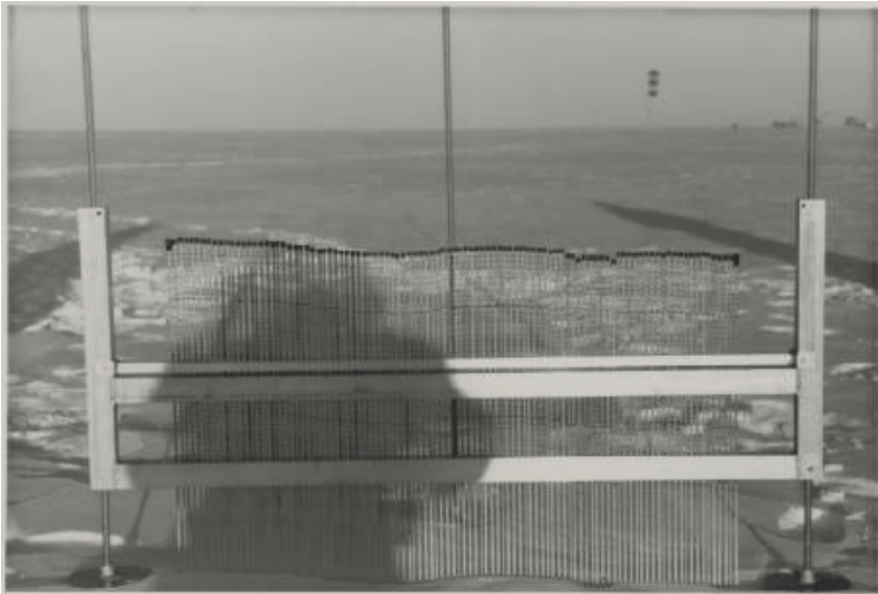
Figure 11. Rods tapped lightly through upper (~1 cm) fresh snow layer. P 28/29 G Book. Measured across wind direction. RMS Height: 0.6 cm; Correlation Length: 7.32 cm
