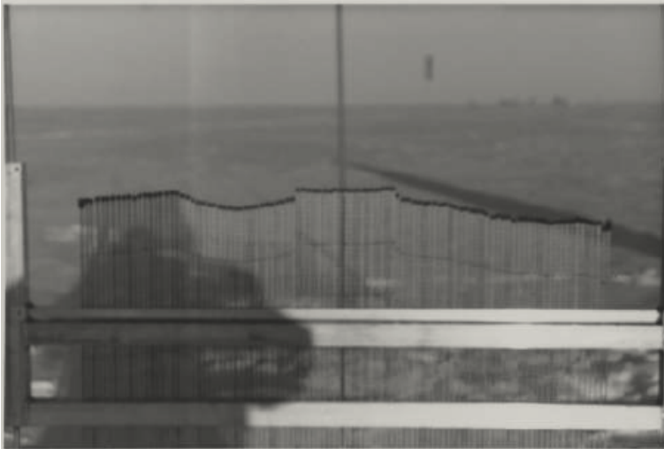
Figure 9. Dune surface measured across wind direction: Page 26/27 G book. RMS Height: 1.57 cm; Correlation Length: 11 cm
