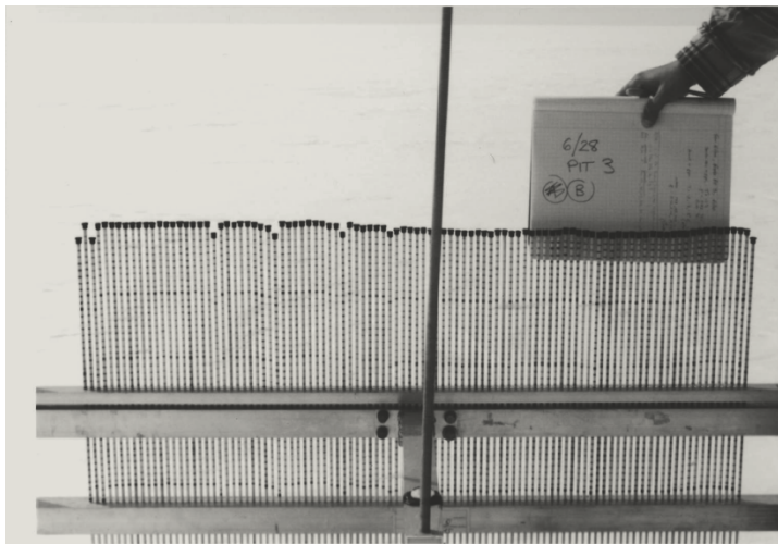
Figure 25. Three, 1-m long measurements of surface roughness. Rod height varies abruptly where the rod falls through the upper thin crust and is stopped by the near surface ice layer. The surface is gently undulating with a peak roughness of less than 2 cm. Upper, middle and lower photos are each displaced by about 1 m along the strike of the gauge.
