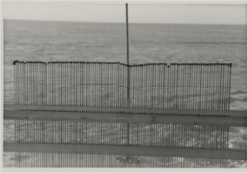
Figure 17. Flat area along dimple shown in figure 9 and along the wind direction. P. 16/17 in G Book. RMS Height: 0.37 cm. Correlation Length 6 cm.
