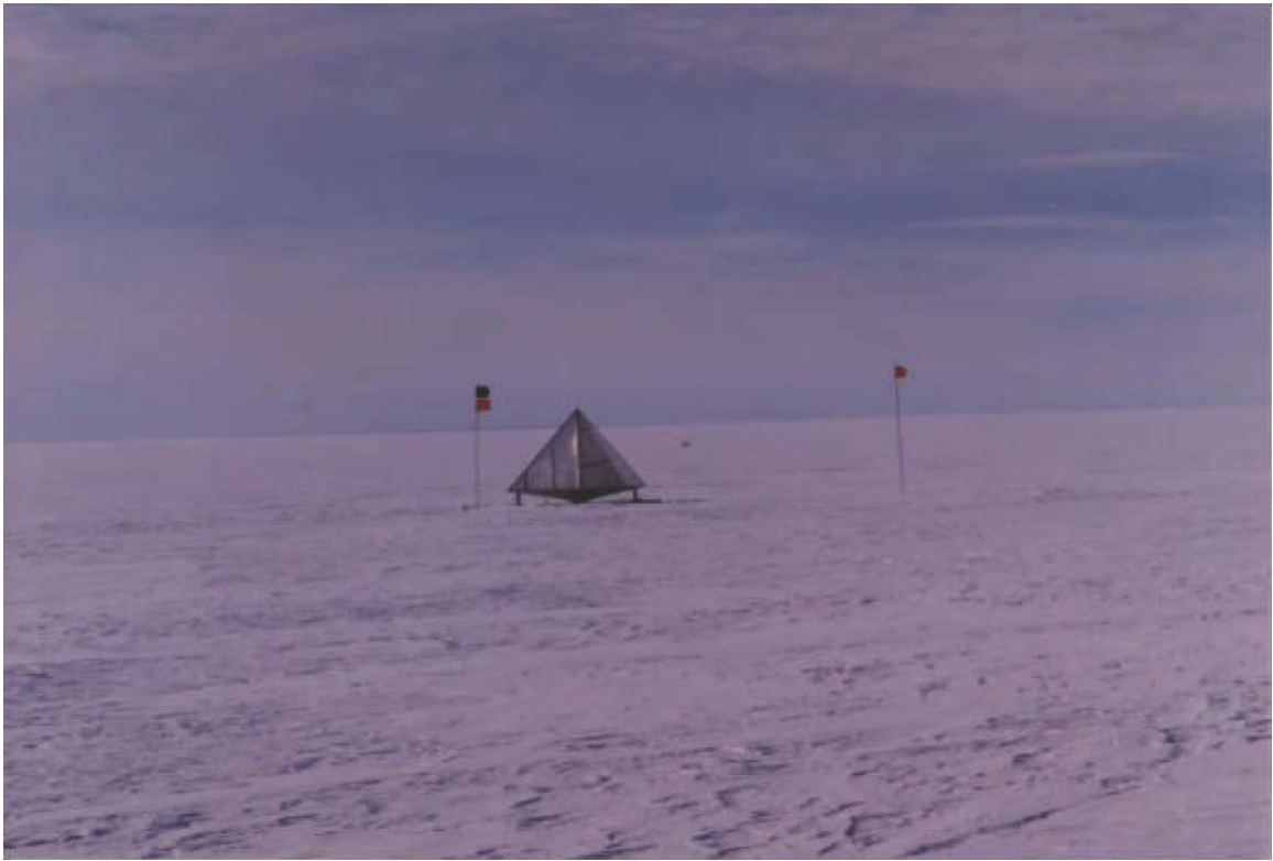
Figure 3. Surface patterns around a 1.5 m corner reflector erected at Crawford Point.
