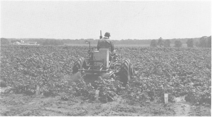
Fig. 3.—Tractor-mounted sprayer unit driven by power take-off on front of motor—also equipped with low-pressure by-pass for application of concentrates.
