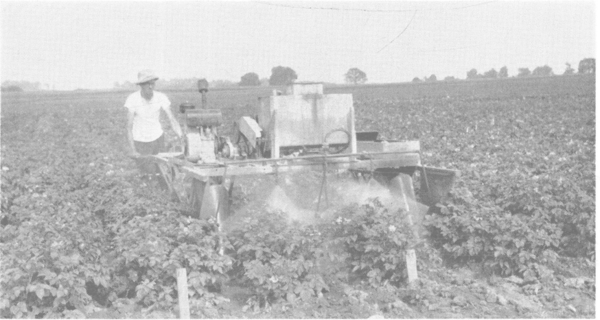
Fig. 1.—Self-propelled sprayer, equipped with speedometer. Capable of very accurate calibration of application rates.
