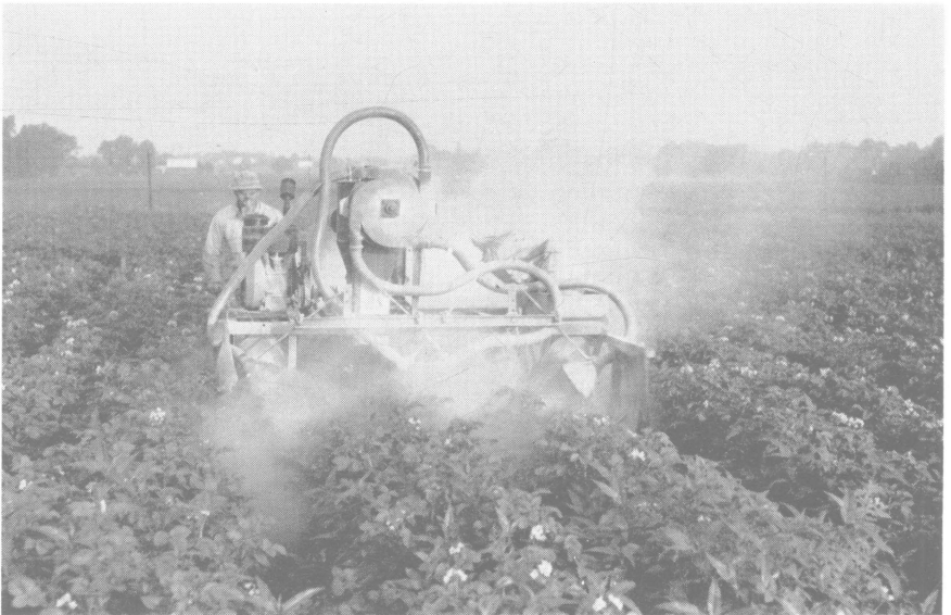
Fig. 2.—Self-propelled duster. Duster hopper equipped with an aerating device, and a special quadrant scale making accurate calibration of flow rates possible.
