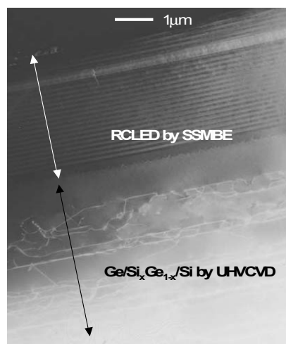
Figure 1. Cross sectional TEM image of a III-V device layer grown on a SiGe substrate.
