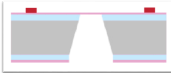
Figure 8: Suspension System after KOH Etching [23]
