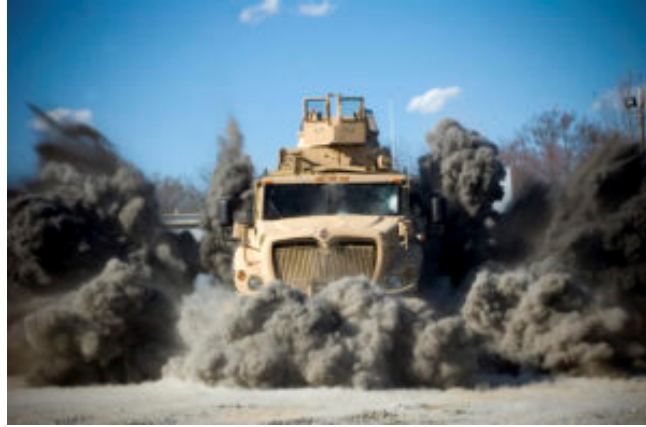
Figure 3: Mine-Resistant Ambush Protected Vehicle (MRAP) being tested with an explosive charge underneath the vehicle. (source: APGnews.com)
