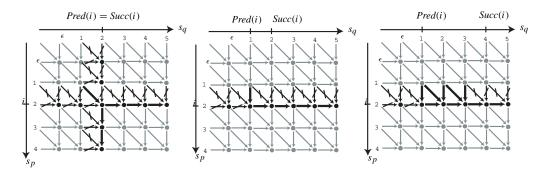
Fig. 3. Three examples of transitivity frontiers for i = 2 in a two dimensional dynamic programming matrix of  $s_p$  and  $s_q$ . Black dots represent cells within the matrix of which incoming edges are affected by the transitivity frontiers considered here.
