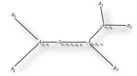
Figure 2.2: A phylogenetic dendrogram to guide the progressive alignment. The input sequences  $\{s_1, s_2, s_3, s_4, s_5\}$  are distributed across the leaves of the tree, and internal nodes represent alignments of respective subsets. Guiding trees are usually unrooted and a further progressive step is necessary to align the partial alignments  $\mathcal{A}_{\{s_1,s_2,s_3\}}$ and  $\mathcal{A}_{\{s_4,s_5\}}$ .
