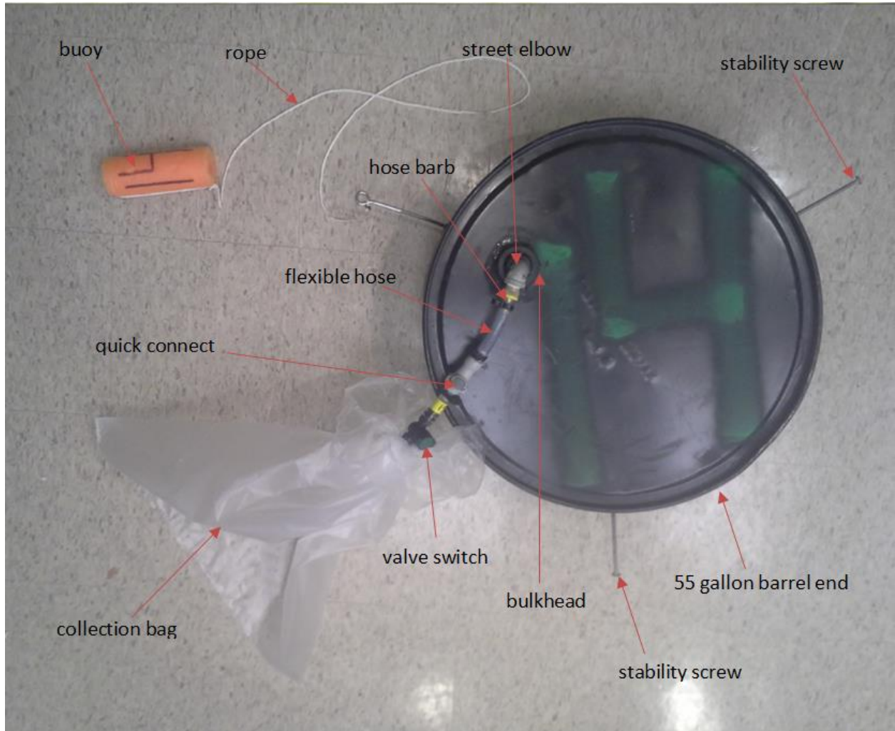
Figure 3. Labeled photograph of a seepage meter.
