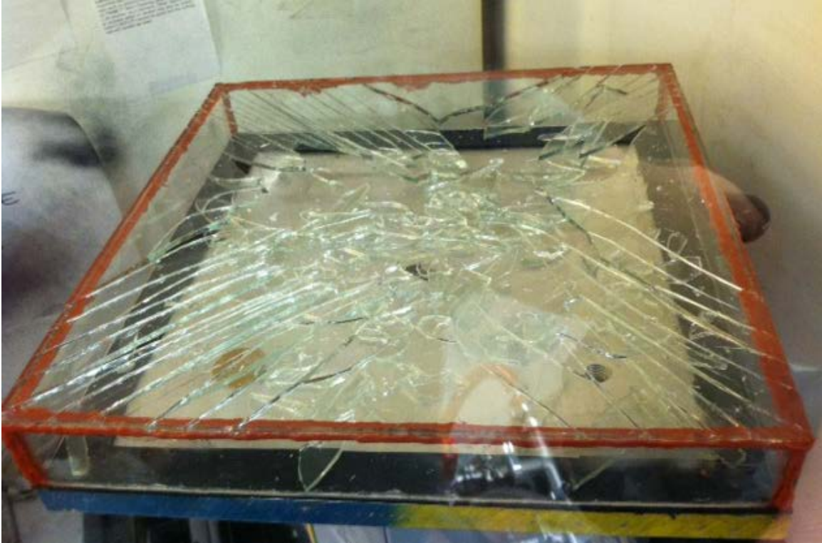
Figure 12: Imploded Chamber after Partial Evacuation
