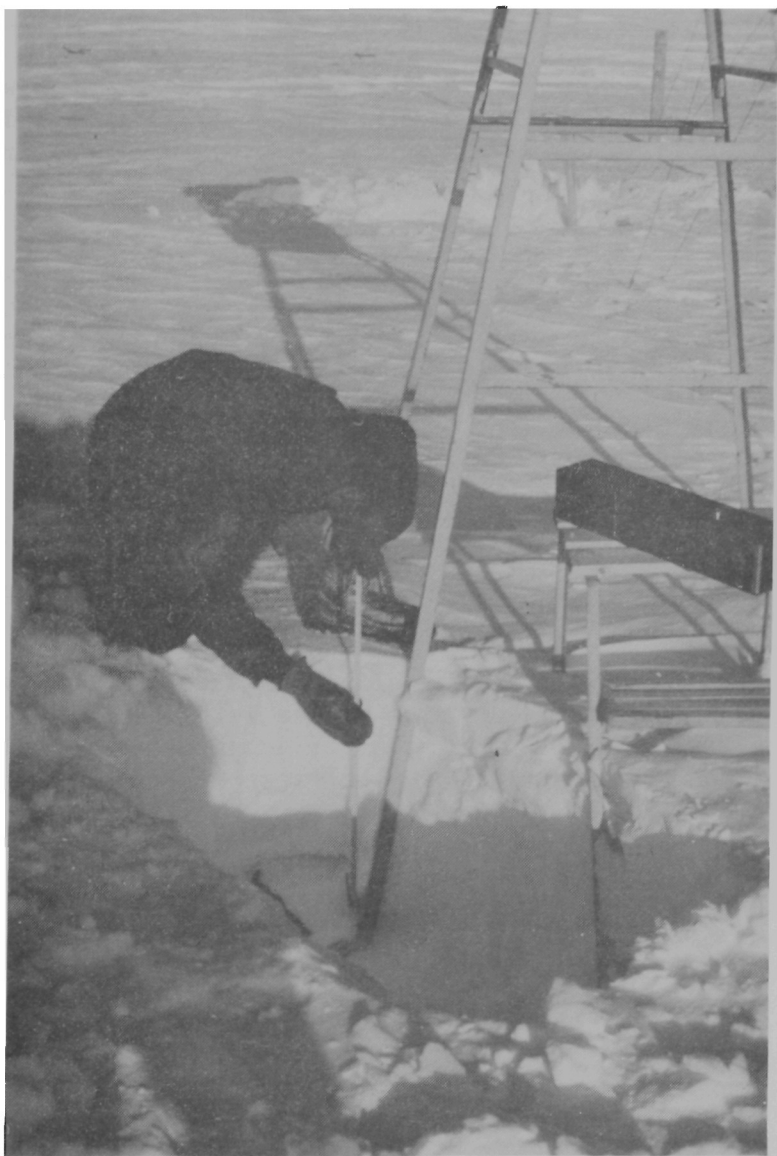
Fig. 31 - Snow accumulation at Pole of Relative Inaccessibility. Measured at meteorological instrument screen; for period 14 December 1958 to 30 January 1965 60 cm of snow ( 3.4 \text{ g/cm}^2 ) (Photo by E. Picciotto)
