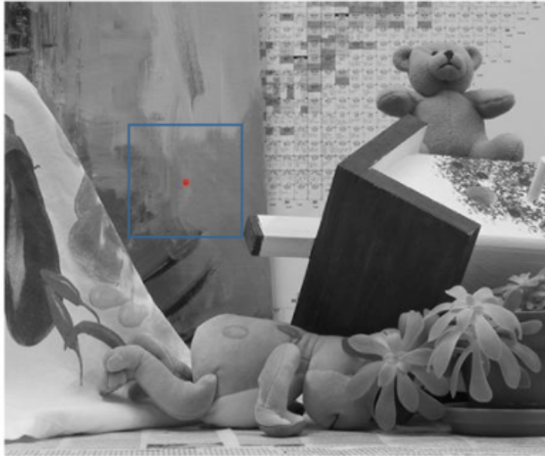
Figure 4. Example of wrong template size which contains not enough strong feature for area-based matching
