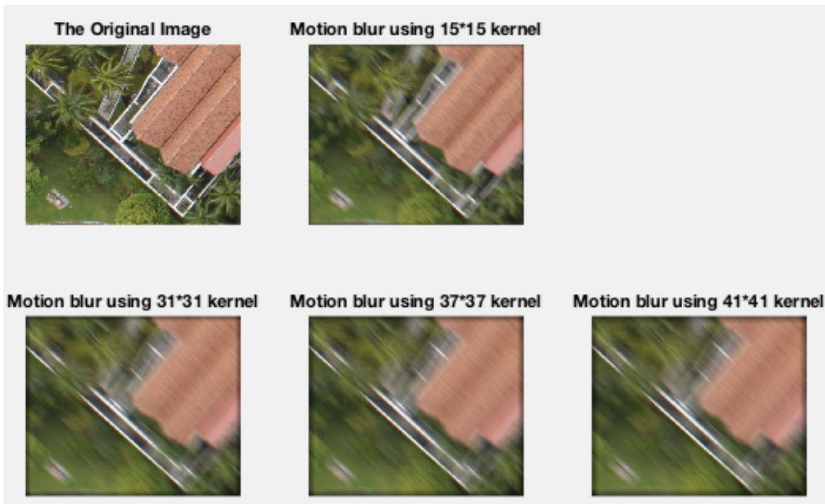
Figure 7. Example of different degrees motion blur images
