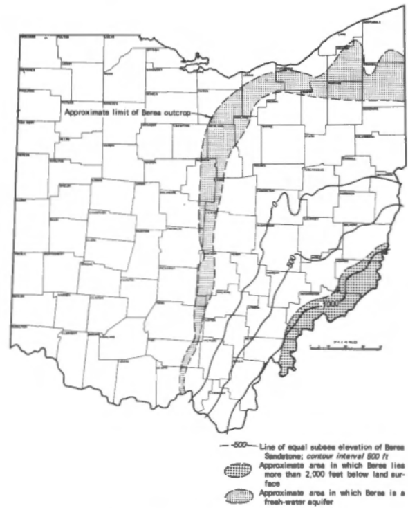
FIGURE 17.—Generalized structure on the Berea Sandstone and locations of deep areas and fresh-water-bearing areas.
