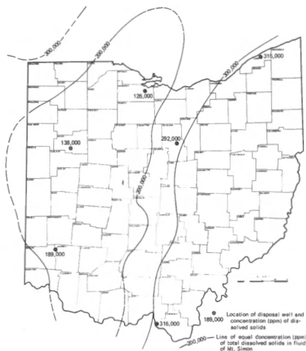
FIGURE 12.—Concentration of total dissolved solids in fluid of the Mt. Simon Sandstone.
