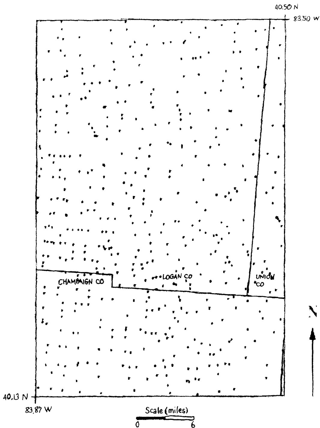
510 geomagnetic and gravity field station locations used in Weaver's survey covering areas of Champaign, Logan, and Union counties. From Weaver (1994)
