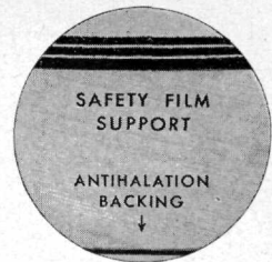
A cross-section of Kodachrome Film showing the extreme thinness of the three color-sensitized coatings separated by plain gelatin layers.
