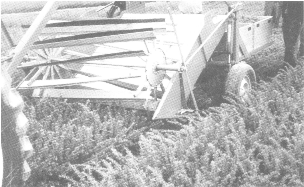
Figure 1. View of Taxus clipping harvester during field operation.
