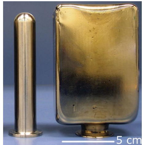
Figure 1.1: Bulk metallic glass formed by blow molding [4].
