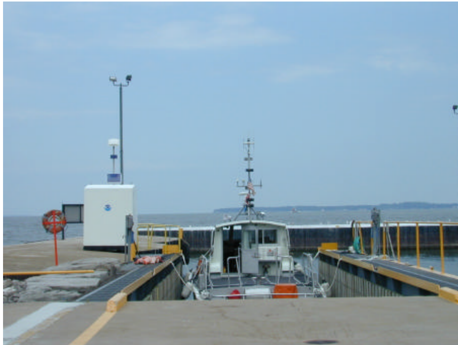
Figure 3.11. The Marblehead tide gauge located in the Marblehead Coast Guard Base. The white box to the left of the boat is the gauge house.
