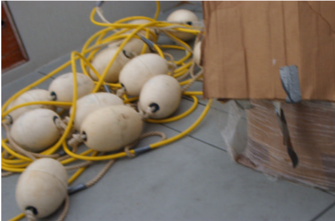
Figure 2.3. The pulling rope and floaters. The rope is taped to a 30 m antenna cable to avoid pulling on the antenna cable while operating.
