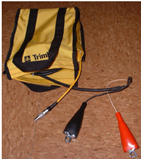
Figure 2.6. The battery pack. The power connectors (black and red) that are able to connect a 12 volt standard automobile battery to the receiver. The yellow silver end goes to the power port of Trimble 4000 SSi receiver.
