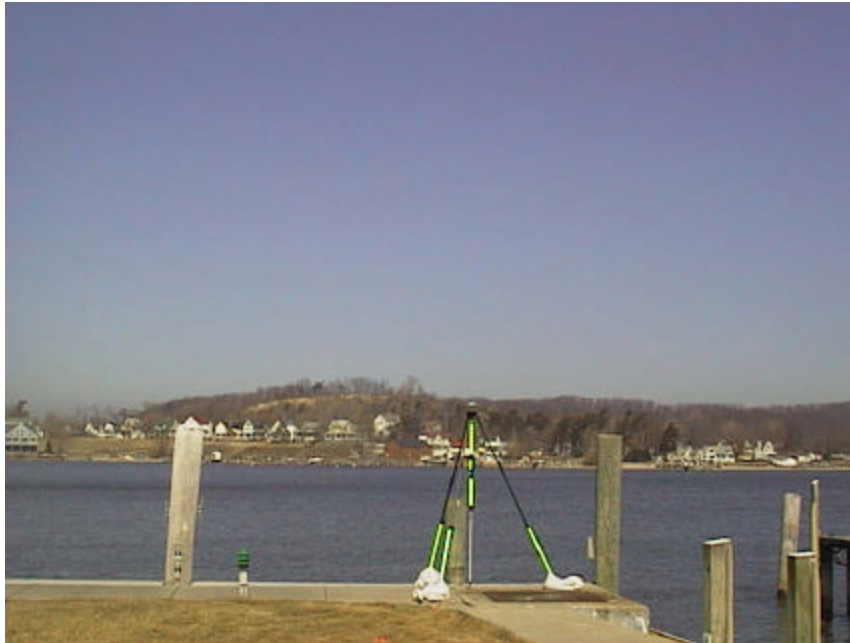
Figure 3.6. The fiducial site at MBYC, close to Holland West tide gauge, was established with the GPS network. The receiver and battery were inside the building.
