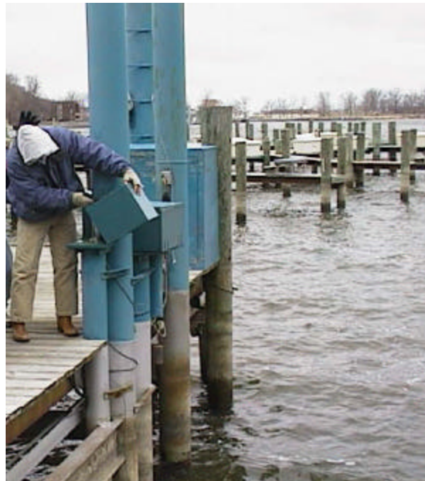
Figure 3.5. The Holland West tide gauge (one of the CO-OPS acoustic sounding gauges in the Great Lakes) producing 6-minute water level continuously.
