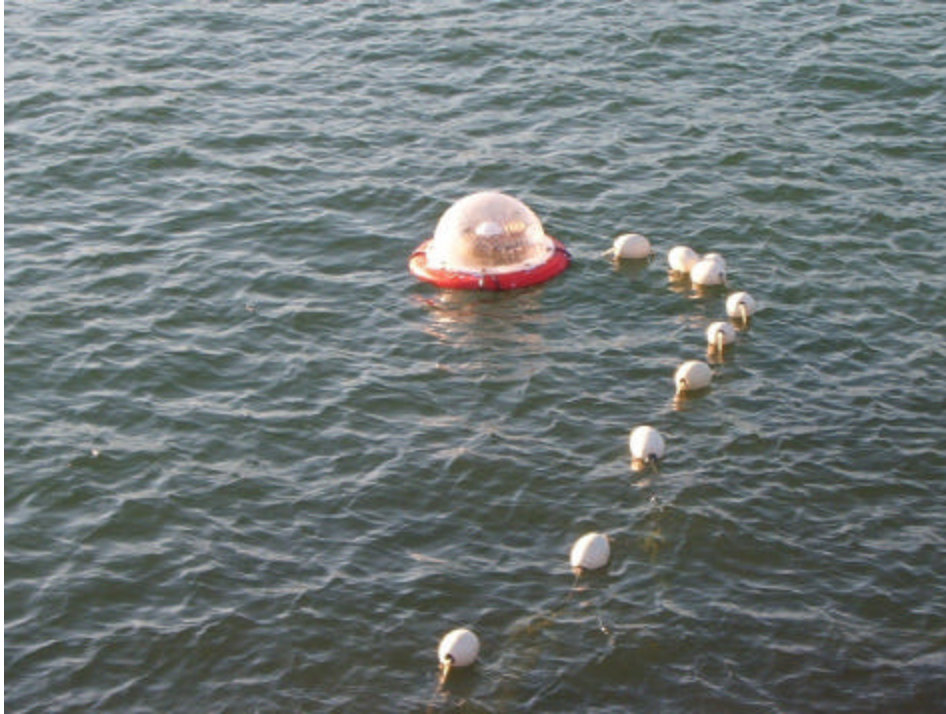
Figure 2.5. Data collection session of the buoy. The yellow antenna cable can be seen underneath the floaters.
